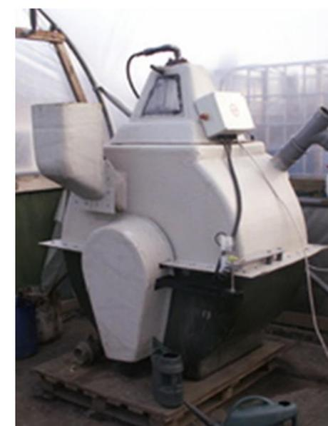
Figure 5. A small scale biodigester
